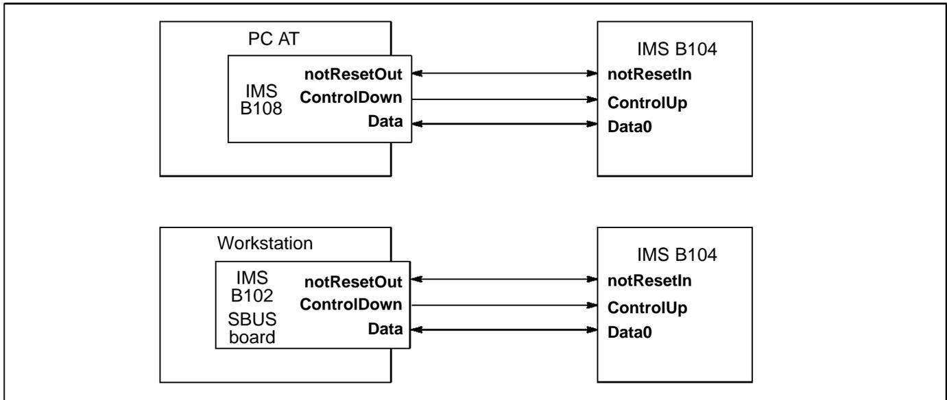
Figure 1.6 Connection to a host interface
