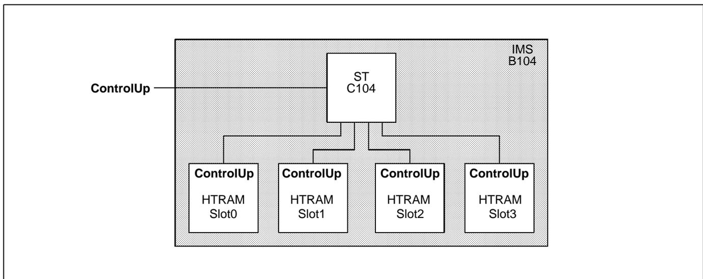
Figure 1.2 HTRAM to ST C104 connection
