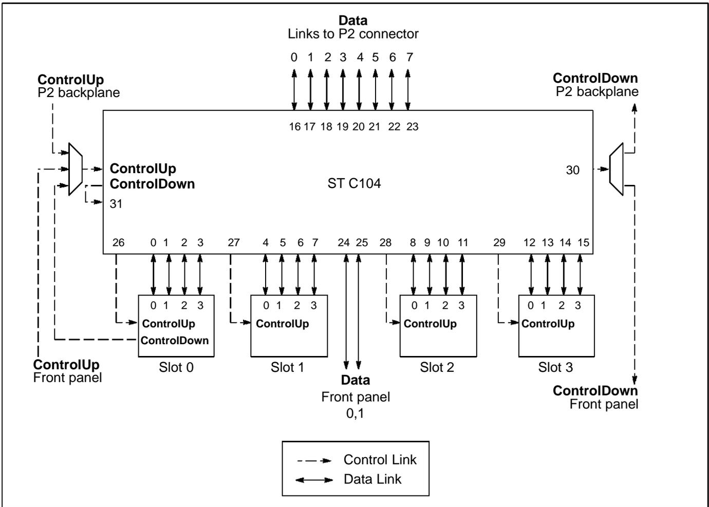
Figure 1.4 Control and data link connections via the ST C104
