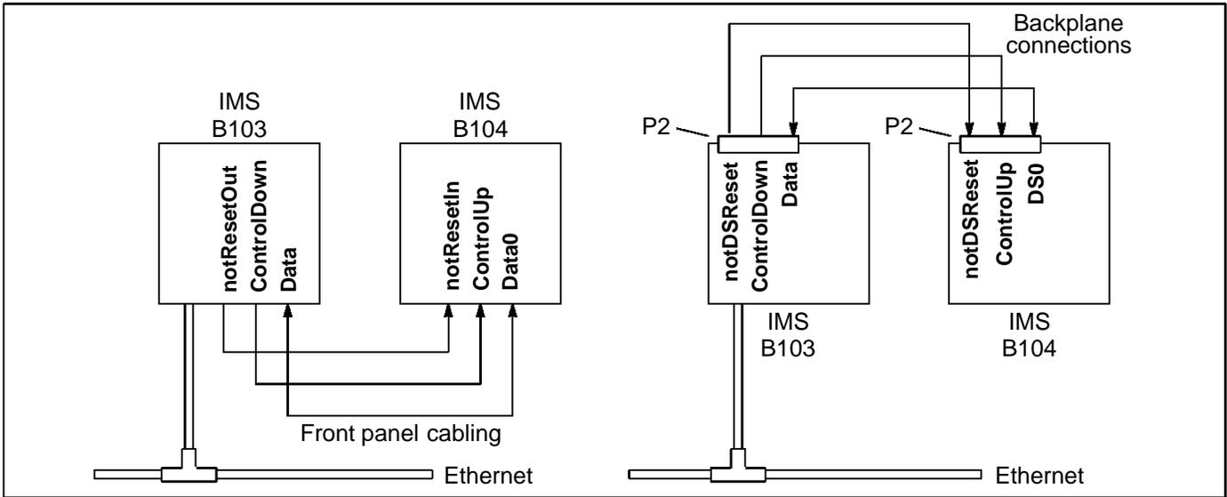
Figure 1.7 Connections to networks of interface boards
